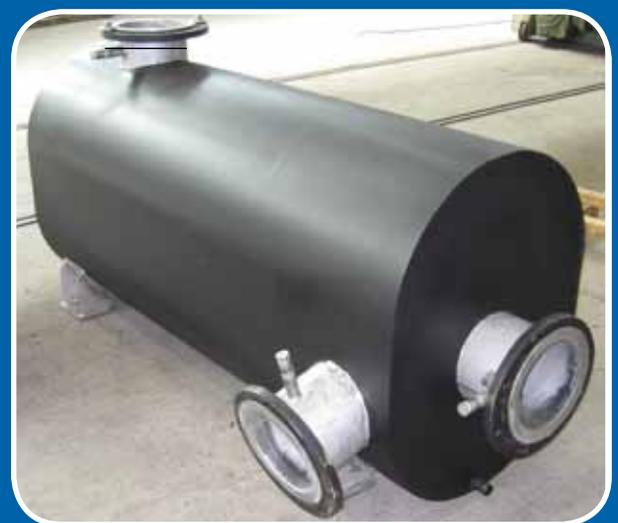
Individual space requirements in the hull of the vessel require individual build layouts for the silencer systems. Nießing can adapt its solutions to fit any situation
