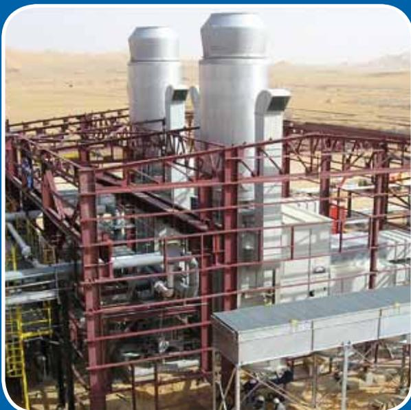
Nießing silencer systems are also used in turbines that are subjected to high temperatures
